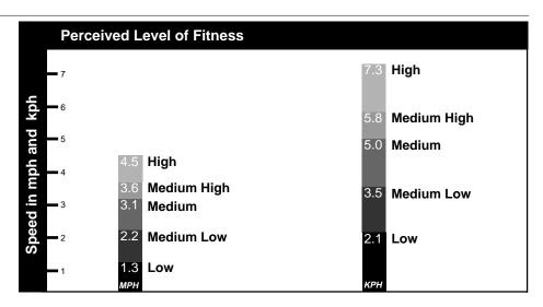
Set the speed of the treadmill based on your perceived level of fitness (low, medium, or high—see Table 1). The incline is preset to accommodate your level of fitness.
